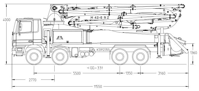
Note: Standard version. Dimensions and weights depend on truck and pump model. Dimensions in mm, MB-Actros 3241 as example
